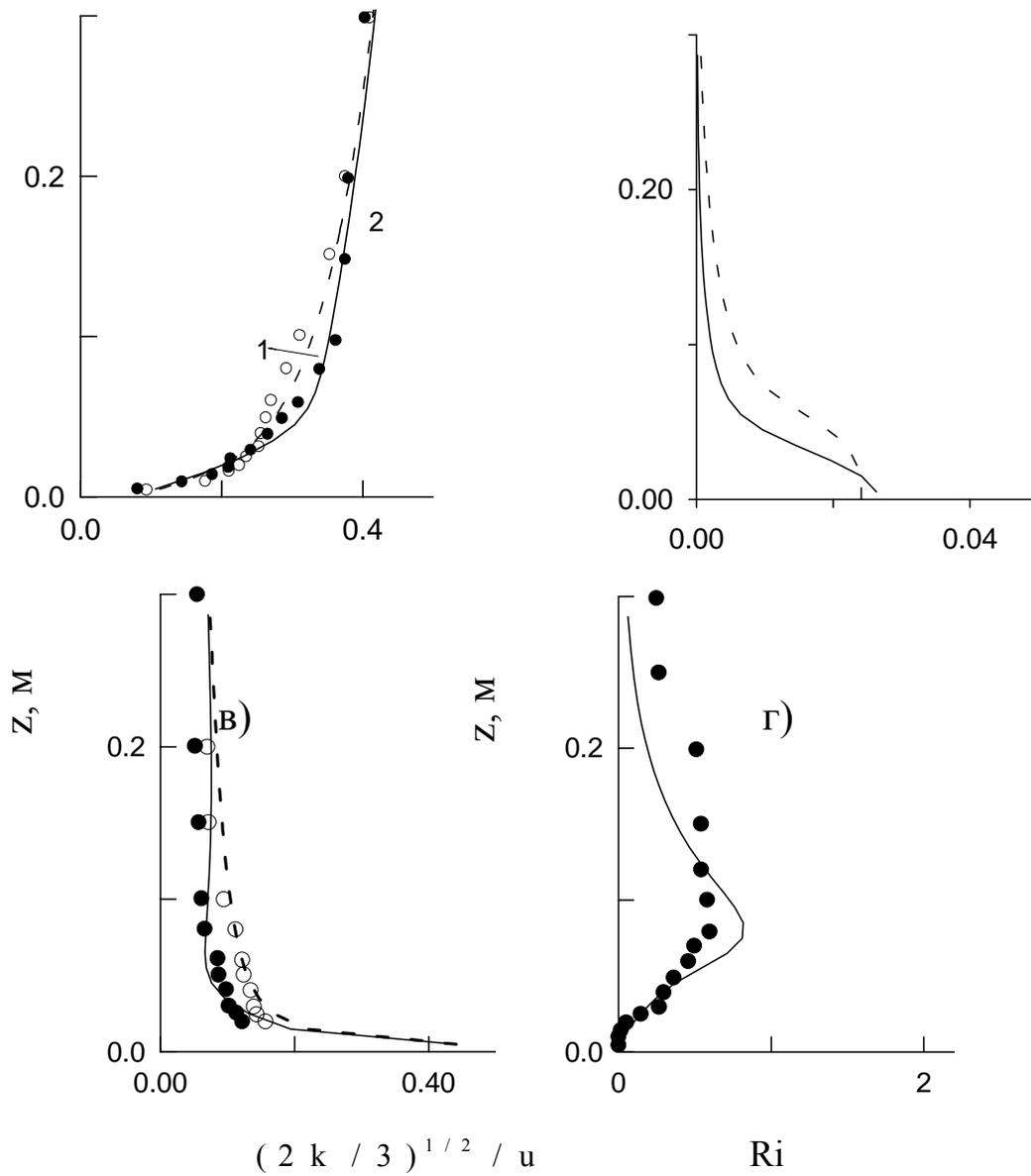
Figure 1 Computed (lines) and measured (circles) vertical profiles of mean velocity (a), concentration (b), energy of turbulence (c) and Richardson number (d) at the distance 2.1 m from source. Solid line and black circle correspond to the heavy gas and dashed line and open circles correspond to the passive scalar.
